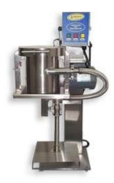
The Hot Disintegrator rapidly and safely removes latency in pulps by recirculating a pulp suspension at an elevated temperature. Disintegrating pulp at elevated temperatures reduces latency by removing the stress that is found in fibres that have been disintegrated at lower temperatures.
